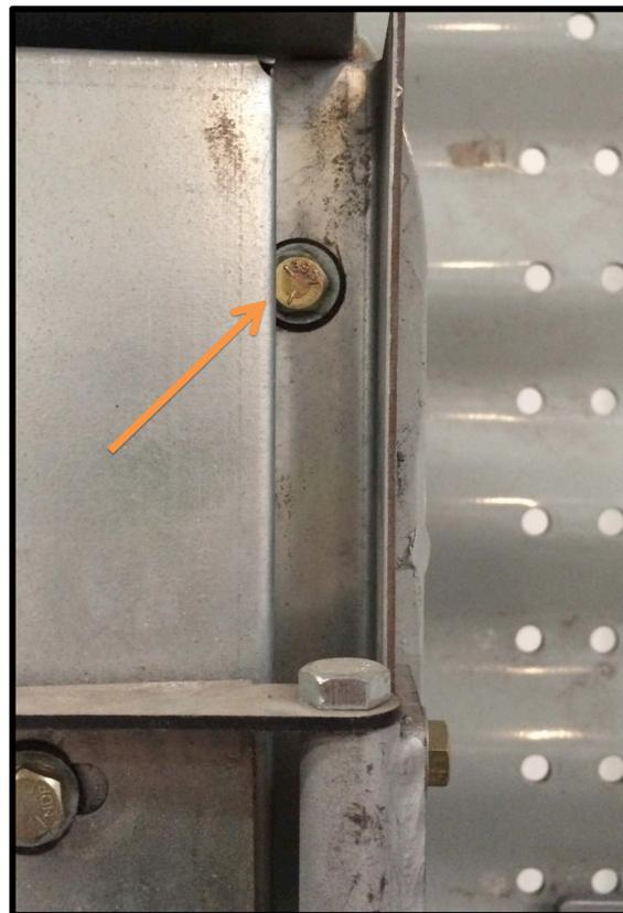
Pictured is a clearance issue with the outer door hitting bolts when closed causing door to be difficult to open/close.
